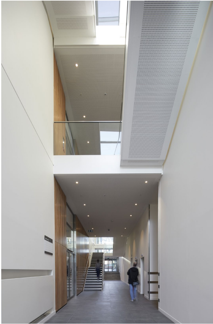
14 View inside The Cut. The 5-storey atrium features European Oak acoustic timber cladding and a full-height stair that links the functions and provides vertical access.
