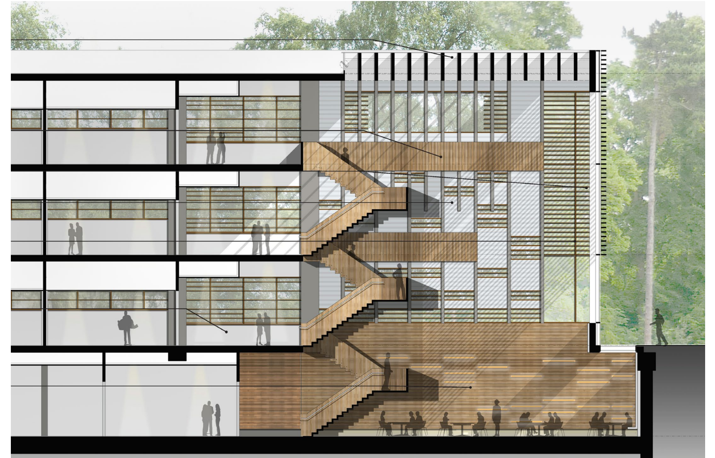
3 Section showing the extent of timber cladding in the atrium and staircase. The interior spaces have been crafted to create an intimate scale and establish a sense of ownership among the research groups that inhabit it.
