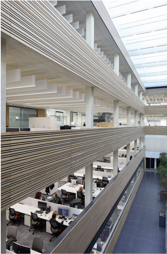
13 View of open-plan working spaces with cellular offices above. The atrium has acoustic timber lining to reduce noise transfer within the open-plan arrangement.
