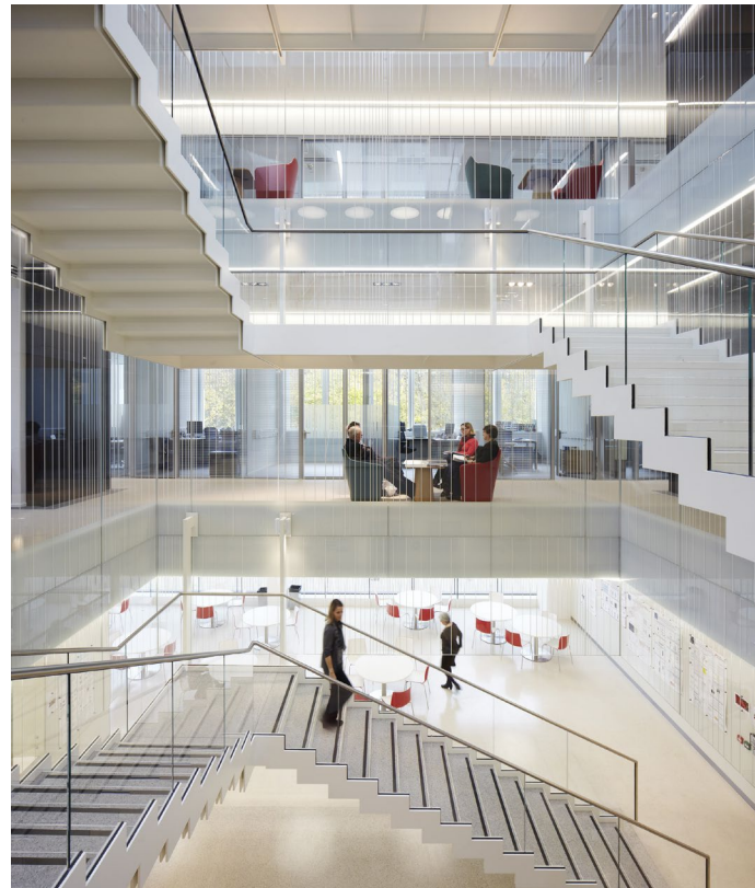
14 (Opposite) First floor views through to the staircase and fabric acoustic wall behind. Thin white fritted stripes emphasise the verticality of the space, while the zig-zagging staircase – formed from steel, terrazzo and glazed balustrades – conveys a crisp sense of precision.
