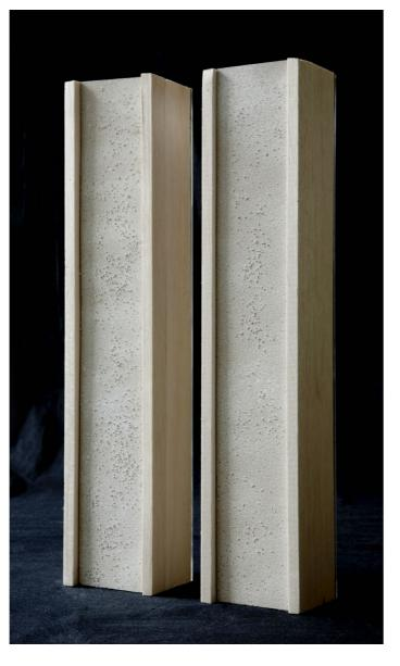
3 Models exploring our innovative straw-bale facade concept, which uses straw in an external curtain wall system. We fitted the straw into timber frames finished with render for a natural look to the external face.
