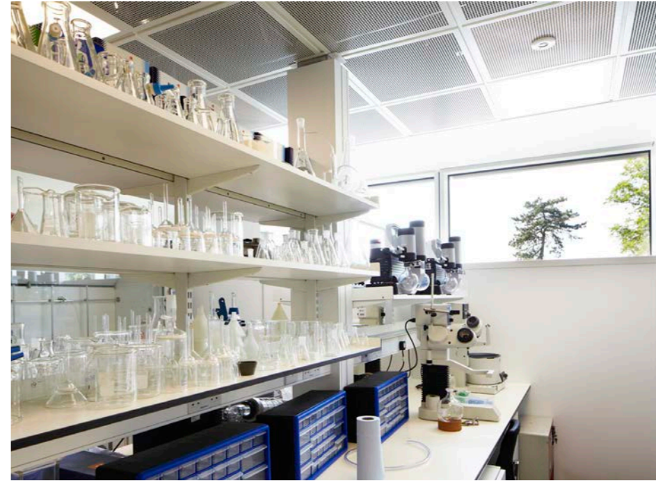
13 Secondary lab with clerestory windows to prevent overlooking.
