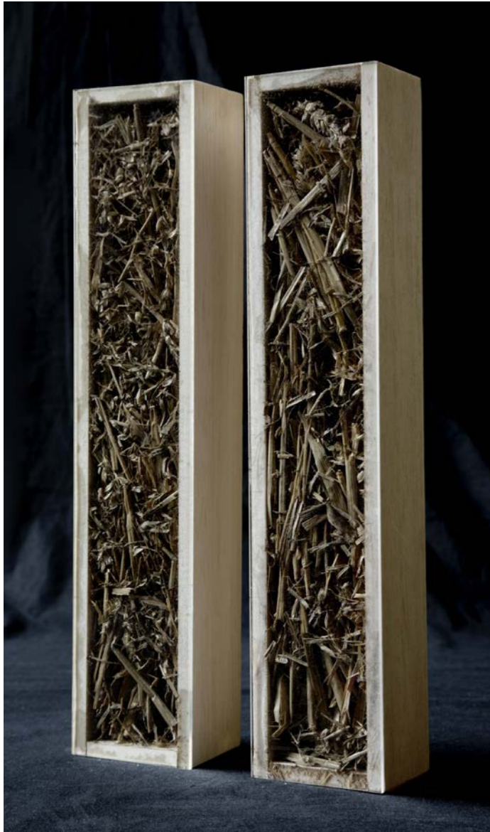
3 Models exploring our innovative straw-bale facade concept, which uses straw in an external curtain wall system. We fitted the straw into timber frames finished with render for a natural look to the external face.
