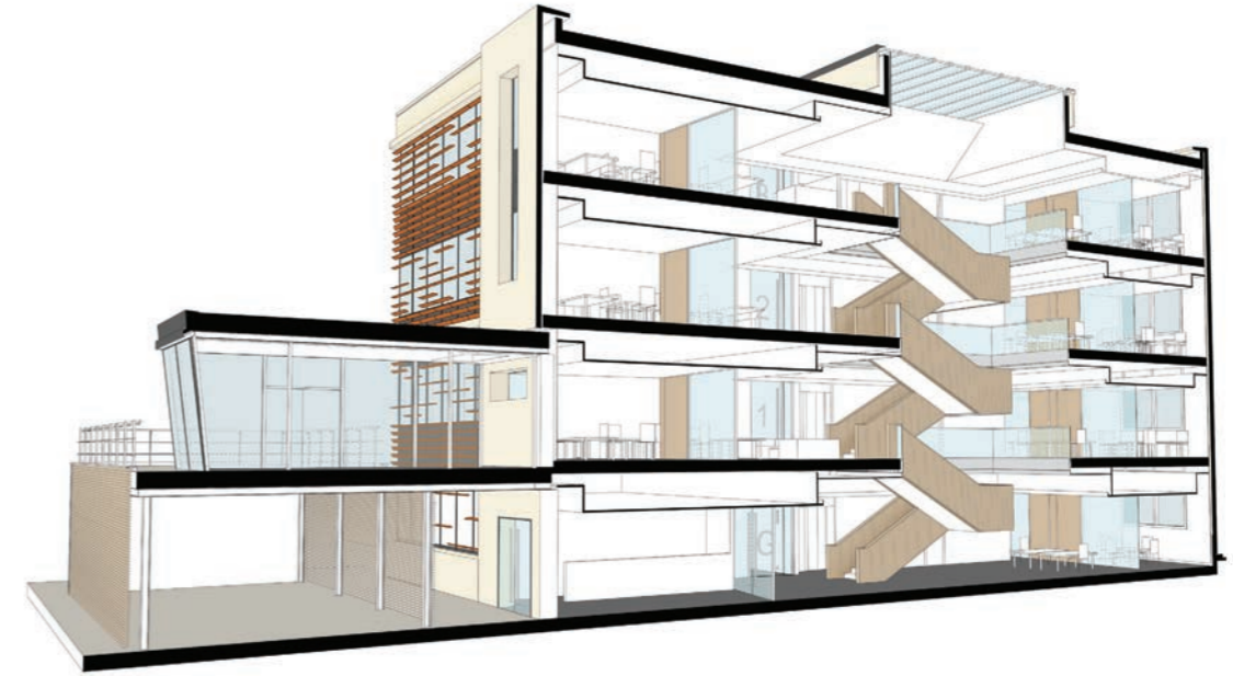
4 Sections showing the top-lit atrium and open-feature staircase. Flexible laboratory spaces surround the stairs, which create a focal point where people can meet and interact.
