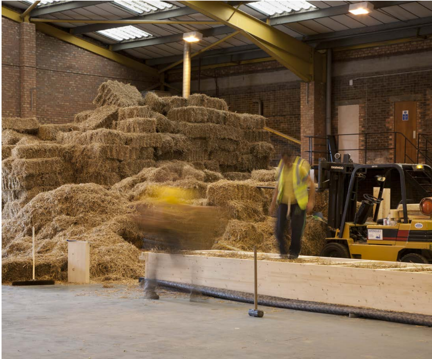
4 The flying factory where the timber panels were prefabricated, using local labour and straw from the university's own farmland – a show of local, sustainable production.
