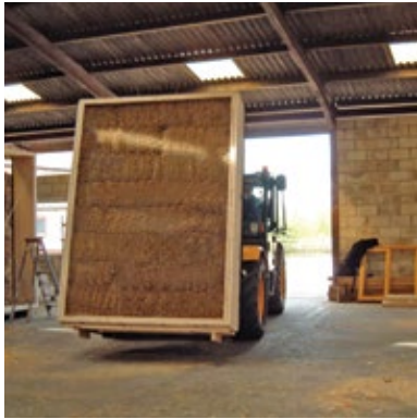
They will be transported to the site and assembled, forming a fully pre-fabricated modular cladding system.
