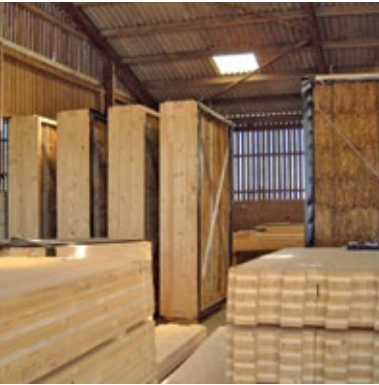
The new bales will then be inserted into the panels and finished with lime render and timber in the 'flying factory' located on the campus.
