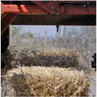
These photos show the straw bale-making process, beginning with the precise trimming of the bales before they are packed and compressed into a timber frame.
